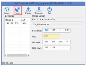
3. Select the device and modify the IP Address or other parameters. Click "Download" button to download configuration to the board.
